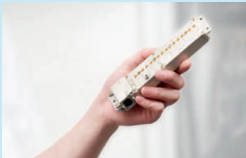
DirectDigital: miniaturized electronics in the coil
