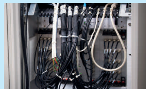
Other MR: Large electronics rack distant from the coil
